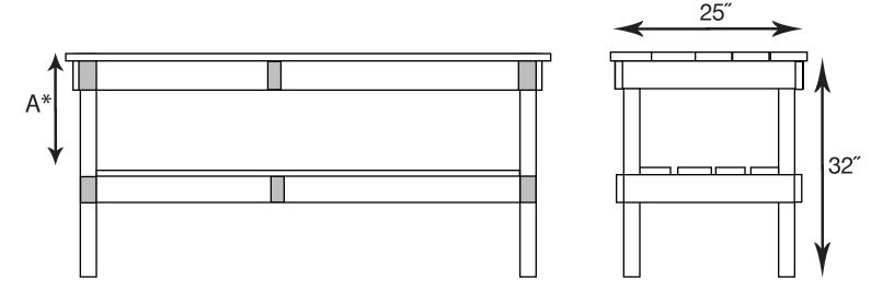
A\* is the measurement from the top of the lower shelf to the table. The "A" measurement is 10"
